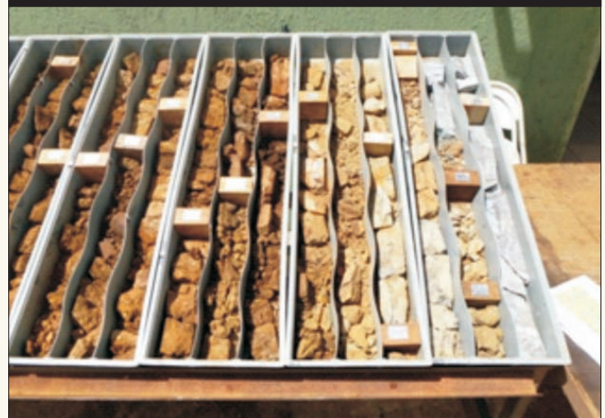
CORE LOGGING - SAPROLITE TO FRESH ROCK BOUNDARY
